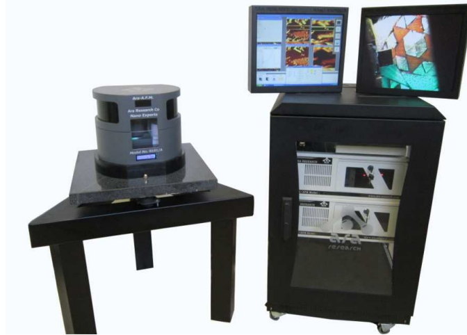
Fig. 1. Atomic Force Microscope made in Iran, modeled ARA-AFM, used in nanomanipulation.
