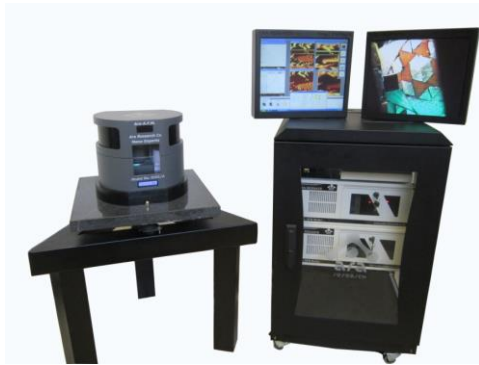
Figure 1: Atomic Force Microscope made in Iran, modeled ARA-AFM, used in Force Spectroscopy.
