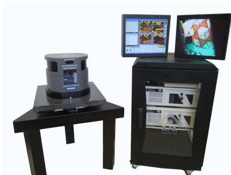
Fig. 4 – Atomic Force Microscope made in Iran, modeled ARA-AFM, used in nanolithography
